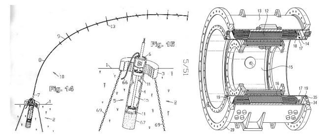
Figure 10 Left: the patent from Selsam.com. Right: Drawing of a new generator module for deep sea (from patent DE 10 2009 034 158 A1 2011.02.03)
