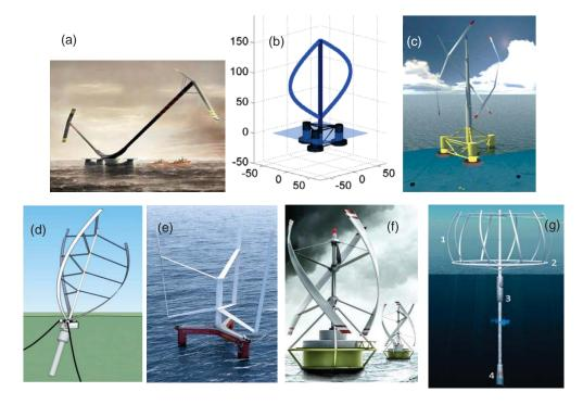
Figure 2 - Other floating VAWT concepts: (a) NOVA semi-submersible; (b) OC4-DeepWind semisubmersible; (c) VertiWind semi-submersible; (d) Floating axis wind turbine; (e) Spinfloat Tri-Floater; (f) Gwind; (g) SeaTwirl
