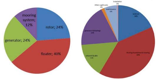
Figure 3 Cost break down of concept: Left-1 unit. Right-20 units in wind farm
