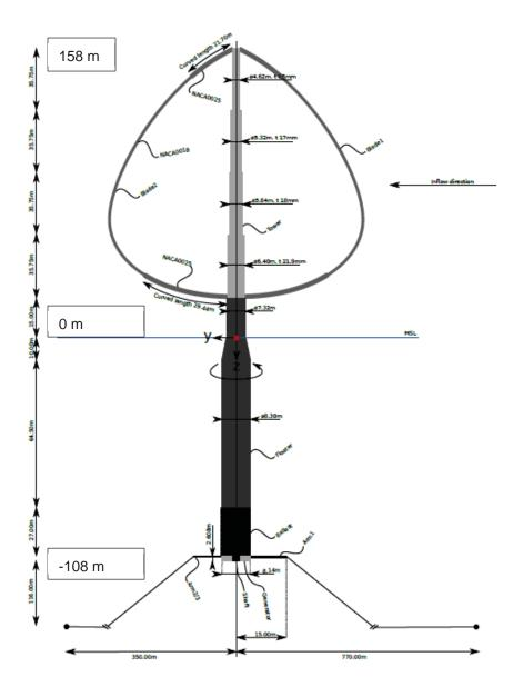
Figure 1 Schematic of the DeepWind concept, obtained from [1]
