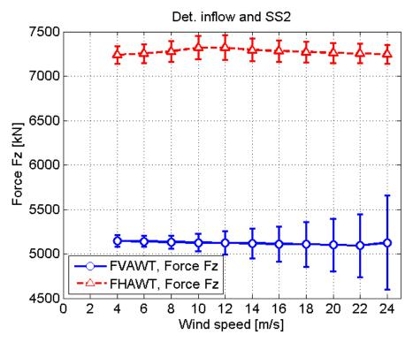
Figure 39 Force Fz at tower bottom for the FVAWT and FHAWT, deterministic inflow, Sea State 2
