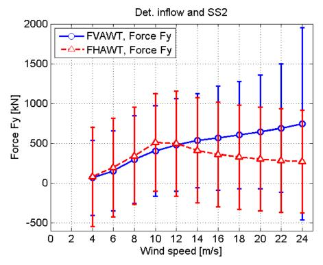
Figure 38 Shear force Fy at tower bottom for the FVAWT and FHAWT, deterministic inflow, Sea State 2
