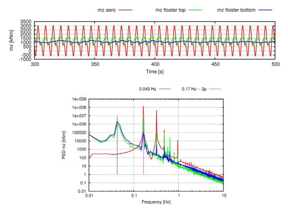
Figure 16 In the upper graph the torque is shown at different positions in the drive train. Below the PSD of the same signals are shown.
