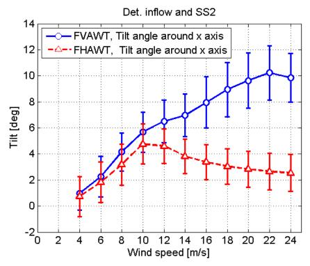
Figure 31 Tilt angle for the FVAWT and FHAWT, deterministic inflow, Sea State 2
