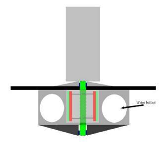
Figure 8 Artistic view of generator module, torque absorption and variable ballast section. The weight of the module can be variable by using pressurized air from a tank inside the floater, and through the hollow generator shaft out in the annulular cavity holding water ballast and hence driving out parts of water, providing a net upward lift.©DTUWE
