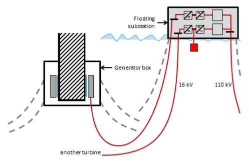
Figure 9 Sketch of Floating turbine and sea station arrangement
