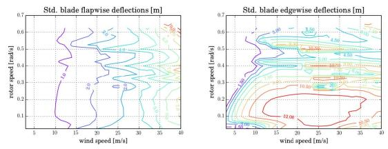
Figure 4 Contour plot of the standard deviation of vibration in the flapwise and edgewise direction of a blade section on the mid part of the rotor as function of rotor speed and wind speed. From D1.3.
