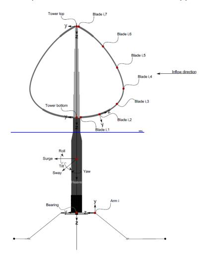
Figure 43 Positions and coordinate systems of the points at which forces, moments and positions
