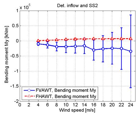
Figure 41 Bending Moment My at tower bottom for the FVAWT and FHAWT, deterministic inflow, Sea State 2
