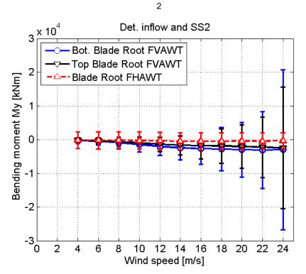
Figure 45 Bend. Moment My at the blade roots for the FVAWT and FHAWT, deterministic inflow, Sea State
