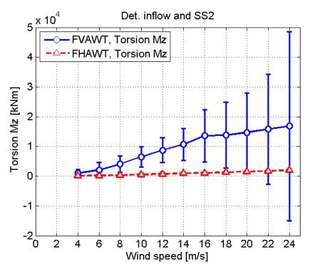
Figure 42 Torsion Mz at tower bottom for the FVAWT and FHAWT, deterministic inflow, Sea State 2
