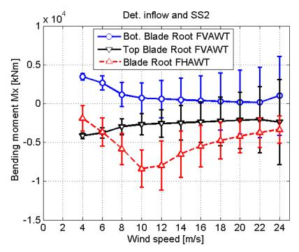
Figure 44 Bend. Moment Mx at the blade roots for the FVAWT and FHAWT, deterministic inflow, Sea State
