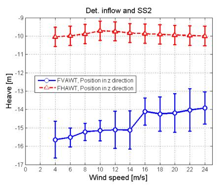
Figure 36 Heave position for the FVAWT and FHAWT, deterministic inflow, Sea State 2
