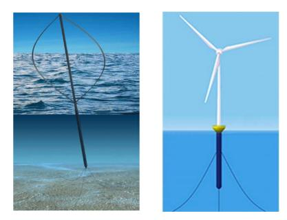
Figure 26 DeepWind 5MW FVAWT (left) and NREL 5MW FHAWT (right) Illustration by: DTU Risø Campus and www.hawc2.dk
