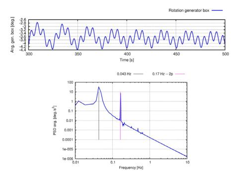
Figure 17 Upper graph shows the rotation of the generator box. The PSD of the same signal is shown in the lower graph.
