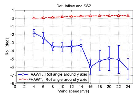
Figure 32 Roll angle for the FVAWT and FHAWT, deterministic inflow, Sea State 2
