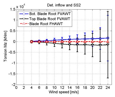
Figure 46 Torsion Mz at the blade roots for the FVAWT and FHAWT, deterministic inflow, Sea State 2
