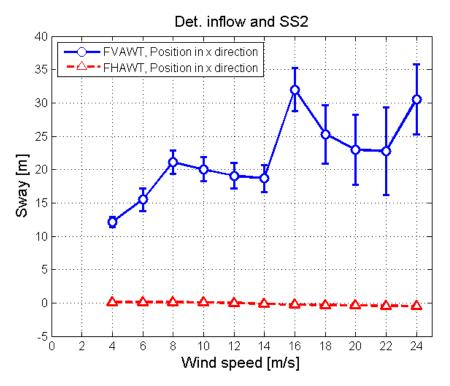
Figure 34 Sway position for the FVAWT and FHAWT, deterministic inflow, Sea State 2
