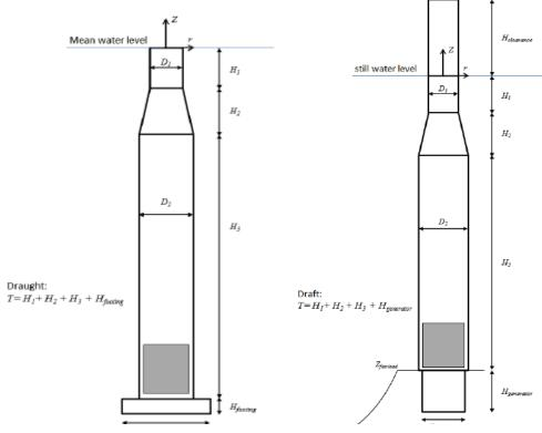
Figure 6 Left: 1<sup>st</sup> iteration design. Right: final floater design
