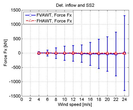
Figure 37 Shear force Fx at tower bottom for the FVAWT and FHAWT, deterministic inflow, Sea State 2
