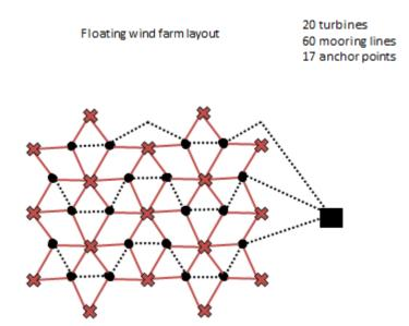
Figure 22 Wind farm layout, saving 33 anchor points out of 60.
