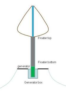
Figure 15 The main components important for the dynamics in the drive train system
