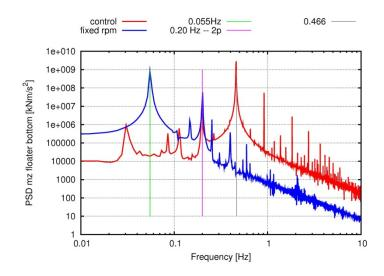
Figure 20 PSD of the torque at the floater bottom for a case at 14m/s with control and with fixed rotational speed, respectively.
