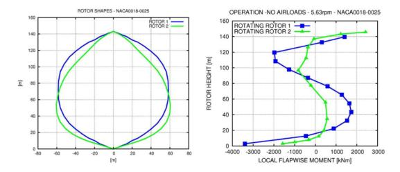
Figure 3 The development of the rotor shape to obtain low mean flapwise bending moments as illustrated by the rotor shape shown in green which was chosen for the final 5MW design.
