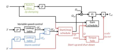
Figure 12 Control for start-up and shut-down
