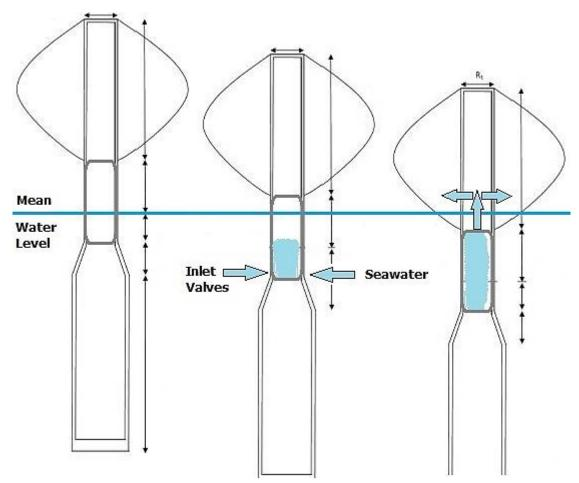
Figure 23 Sketch of the concept showing stages of the braking[8.]
