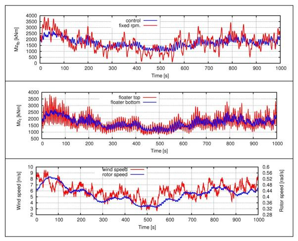
Figure 18 Upper graph shows the torque at the bottom of the floater with control and with fixed rpm, respectively. In the middle graph the toque at the top and bottom of the floater, respectively is compared for the case with control. Finally the rotational speed and the wind speed is shown in the lower graph.
