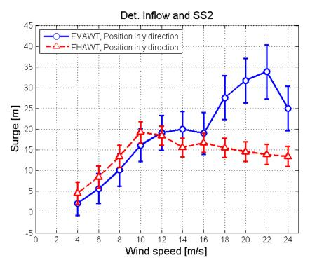
Figure 35 Surge position for the FVAWT and FHAWT, deterministic inflow, Sea State 2
