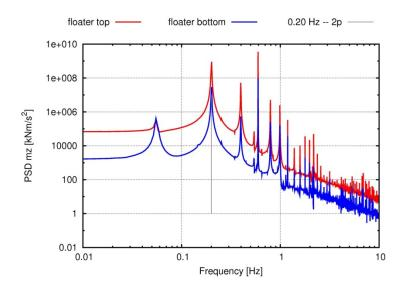
Figure 21 PSD of the torque in the top and bottom of the floater for a wind speed of 14m/s and fixed rotational speed.
