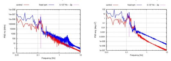
Figure 19 To the left is shown the PSD of the torque in the bottom of the floater for the control and fixed rpm case, respectively. To the right is shown the PSD of the angular rotation for the same two cases.
