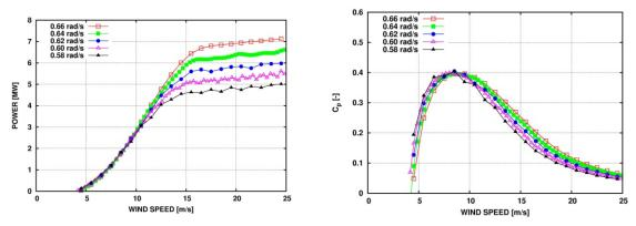
Figure 5 The mechanical power curves for the rotor for different rotational speed are shown in the left figure. To the right is the local power coefficient.
