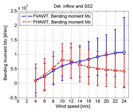
Figure 40 Bending Moment Mx at tower bottom for the FVAWT and FHAWT, deterministic inflow, Sea State 2
