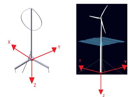
Figure 30. Global coordinate system for the FVAWT and the FHAWT
