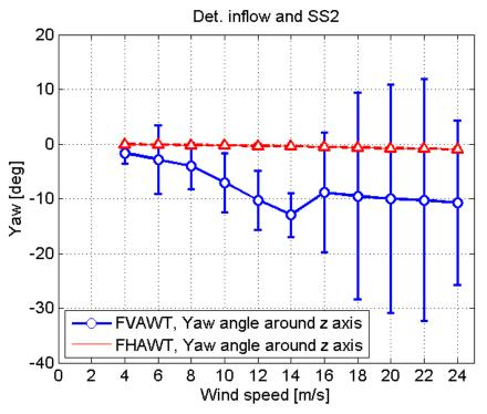
Figure 33 Yaw angle for the FVAWT and FHAWT, deterministic inflow, Sea State 2
