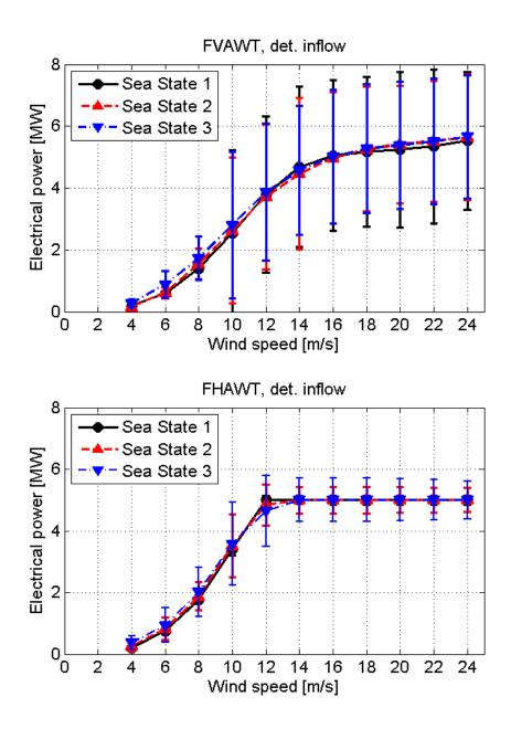
Figure 27 Power curves for the FVAWT Deepwind 5MW and the FHAWT NREL 5MW with deterministic inflow
