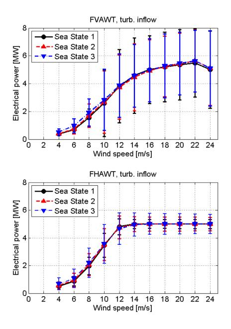
Figure 28 Power curves for the FVAWT Deepwind 5MW and the FHAWT NREL 5MW with turbulent inflow
