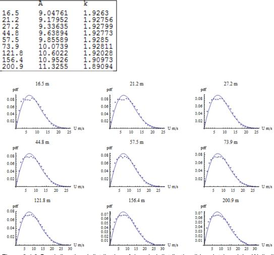
Figure 3.4.1 The Weibull scale and shape parameters A (m/s) and k from WRF data at 9 heights as indicated in the first column.
