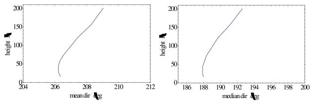
Figure 3.4.11. Vertical distribution of mean wind direction up to 200 m (left) and median wind direction (right), data are from the WRF simulation.
