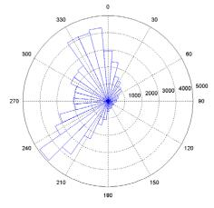
Figure 2.3.3. Wind Rose, wind direction distribution, with number of occurrences on the radial axis, from the IJmuiden data [1].
