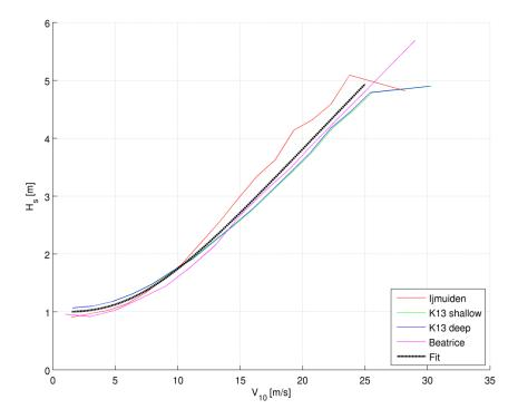
Figure 2.4.5 H<sub>S</sub> versus the 10 meter wind speed for the 4 sites considered with wave measurements. The H<sub>S</sub> values for the fifth site were estimated from wave models only and are not shown here. The fit is defined as  $H_S/H_0 = 1 + 2.6 (V/V_0)^3/(1+(V/V_0)^2)$ , with  $H_0 = 1m$  and  $V_0 = 13 m/s$ .
