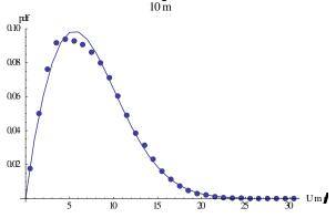
Figure 3.4.4 Omni-directional distribution of the wind distribution (blue dots) and the Weibull fitting of the CSFR 10 m winds, with A=8.836 m/s and k=1.87
