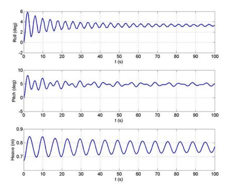
Figure 4.7.11 The 3-DOF of demonstrator during no wind, waves or currents
