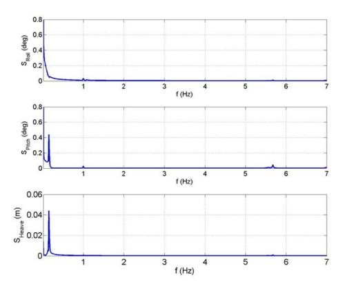
Figure 4.7.13 The three degrees of freedom of the demonstrator as function of frequency. Wind and waves are present and the shaft is rotating.
