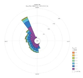
Figure 3.2.5 Wind rose of the wave directions and the directions probabilities of occurrence as function of the significant wave height ( $H_{m0}$  in the figure).
