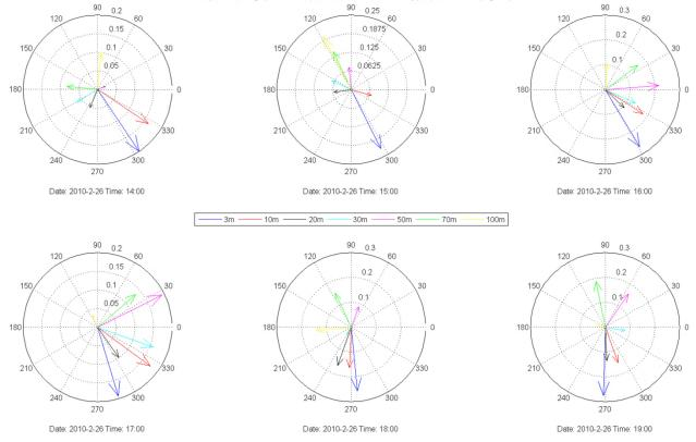
Figure 3.3.3 Series of polar plots depicting depth and temporal variation of current with water depth over six hours, from 1400-1900. Measurement from Utsira. The depths are indicated by colour in the 3-100 meter interval.
