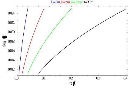
Figure 4.6.3 Heave frequency as a function of slenderness for different hull diameter
