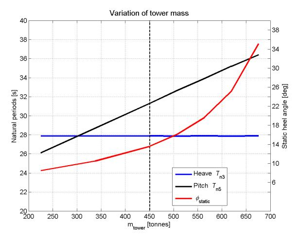
Figure 5.3.3 Effect of variation of tower mass on natural period and tilt angle
