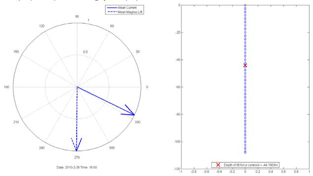
Figure 3.3.8 Normalised Mean Currents and Global Magnus Lift Force for 3 1-hour periods(2/3)
