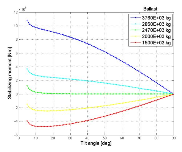
Figure 5.2.3 Moment of stability to counteract, for use of different sets of ballast to maintain a tilt angle.
