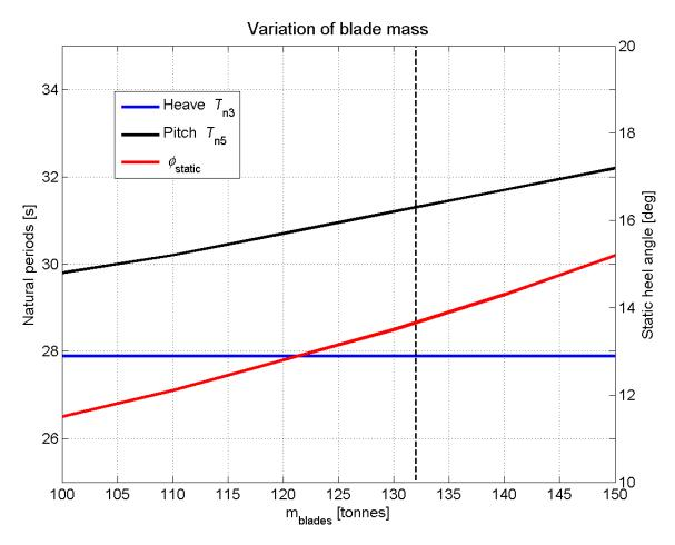
Figure 5.3.2 Effect of variation of blade mass on natural period and tilt angle
