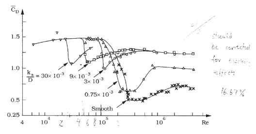
Figure 4.7.4 Drag coefficient of a circular cylinder at various surface roughness's parameters k<sub>s</sub>/D. [[76.]]
