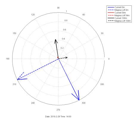
Figure 3.3.4 Normalised Local Currents and Magnus Lift Forces at 0, 54 and 108 m depths for three 1-hour periods (1/3)
