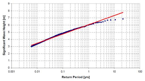
Figure 2.3.8. Extreme  $H_s$  versus return period by the Gumbel method for the K13 shallow depth site of UpWind. From [1].
