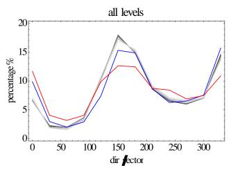
Figure 3.4.6. Wind direction distribution in 12 sectors. The black-gray lines are the WRF data (black at 16.7 m and gray at high level, grayer at higher level). The blue curve is the CFSR data. The red curve is the measurements from Utsira.
