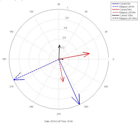
Figure 3.3.5 Normalised Local Currents and Magnus Lift Forces at 0, 54 and 108 m depths for 3 1-hour periods (2/3)
