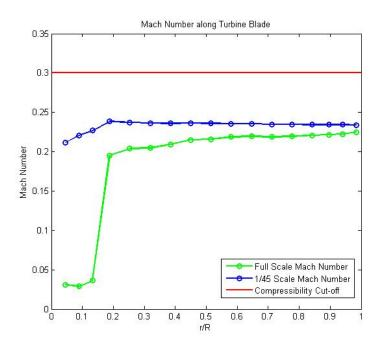
Figure 3.1.1. Mach number calculation for a full scale NREL 5 MW reference turbine and its  $1/45^{th}$  scale model (calculated using BEM theory) [29]. The Mach numbers in both systems are below 0.3, which validates the assumption of incompressible flow at full and model scales. This data was generated in a simulation where the wind speed was 11.4 m/s and the rotor *TSR* was 6.958.
