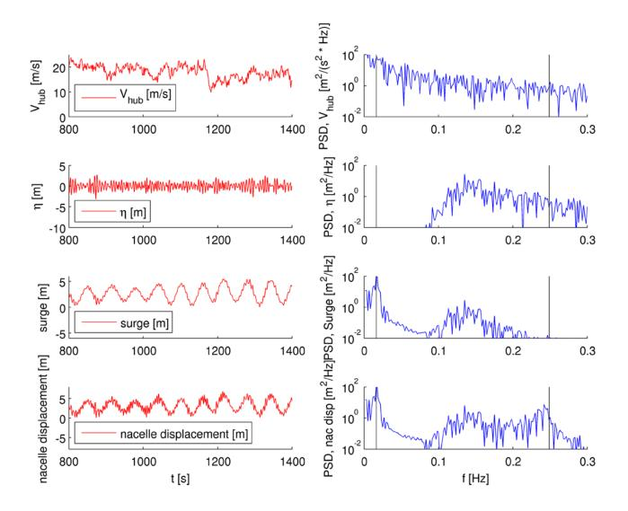
Figure 3.4.3. Response at prototype scale for simultaneous wind and wave loading.
