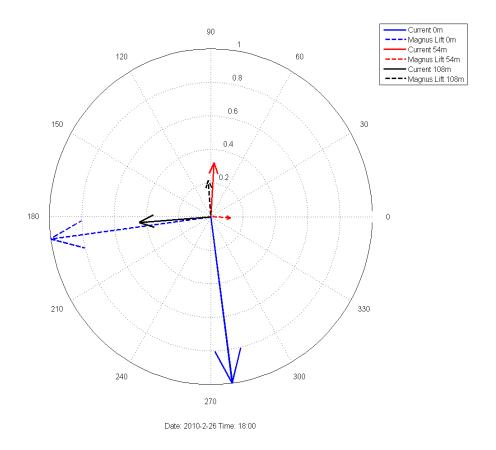
Figure 3.3.6 Normalised Local Currents and Magnus Lift Forces at 0, 54 and 108 m depths for 3 1-hour periods (3/3)
