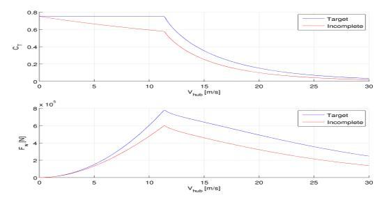
Figure 3.4.5. Consequences of imperfect aerodynamic scaling: Left: Imperfect aerodynamic thrust curve and target thrust curve. Right: Comparison of prototype scale response and model scale response. The model-scale response was produced with the imperfect thrust curve and scaled back to proto-type scale.
