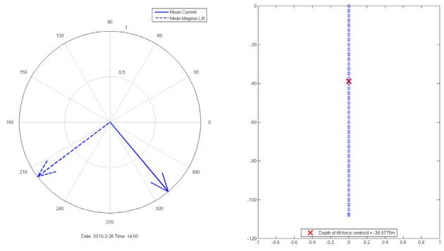
Figure 3.3.7 Normalised Mean Currents and Global Magnus Lift Force for 3 1-hour periods, averaged over the depth (0-108m) of the rotating cylinder (1/3)
