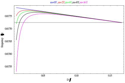
Figure 4.6.2 Influence of ballast weight on heave frequency with the geometric ratio of D/L
