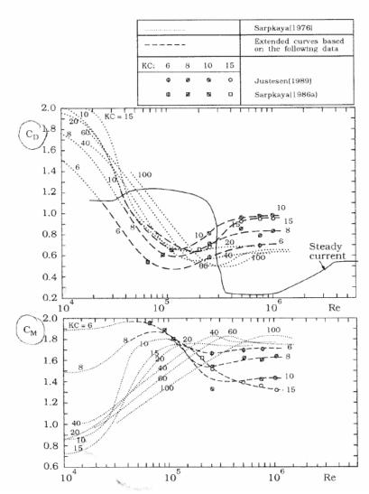
Figure 4.7.6 In line force coefficients for a free, smooth cylinder[[77.]]
