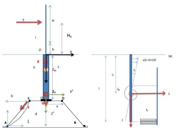
Figure 4.6.1 3-DOF Model of the DeepWind rotor, floater and mooring system
