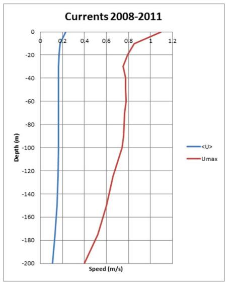
Figure 3.3.1 Measured average speed and maximum speed of water current at Karmøy
