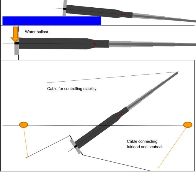
Figure 5.2.5 Installation steps for DeepWind
