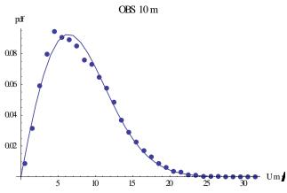
Figure 3.4.5. Omni-directional distribution of the wind distribution (blue dots) at Utsira and the Weibull fitting of the measured 10 m winds, with A=9.16 m/s and k=1.96.
