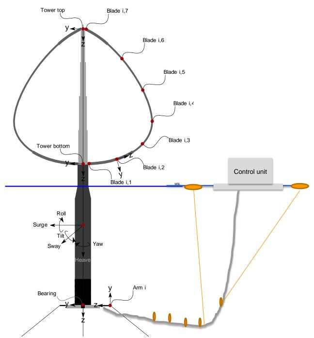
Figure 5.1.3 Left: Sketch of the overall 5MW DeepWind concept[[65.]].Right: Power cable and controller facility Courtesy DTU
