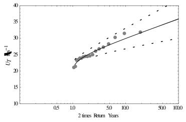
Figure 3.4.13. T-year return wind distribution from 10 -m measurements from Utsira. The basis period of 6 months was used, so that 100 on the x-axis corresponds to 50-year.
