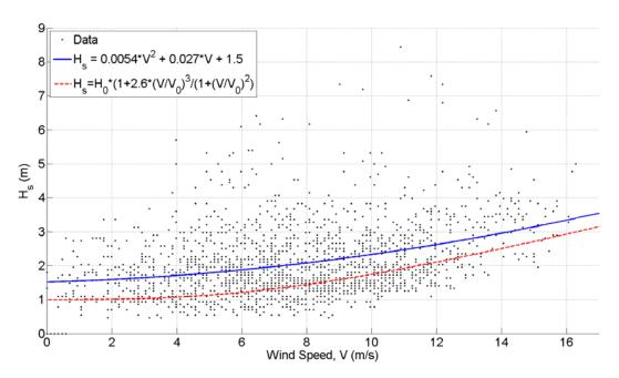
Figure 3.2.8 Hs versus the 10 meter wind speed for the Demo-site considered with wave measurements. The  $H_s$  values for the site are fitted with a quadratic fit as shown in the plot. Also the function presented (2.4.1) and used in Figure 2.4.5 is shown for comparison and us.
