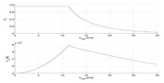
Figure 3.4.2. Thrust coefficient and thrust as function of inflow speed V.
