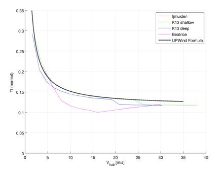
Figure 2.4.4 Normal turbulence intensity versus wind speed at the hub height from 4 of the sites considered. The black curve is the normal turbulence formula from [1] given in (2.3.5), which is the basis for the TI estimates from the UpWind sites. The Beatrice TI is determined from TI values over the North Sea extrapolated by use of (2.3.3). No independent TI was estimated at the fifth site.
