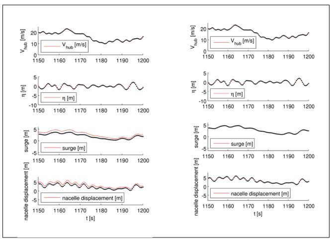
Figure 3.4.4. Comparison of prototype scale results (red line) and model scale results (black dots). The model scale results have been scaled up to prototype scale before plotting.
