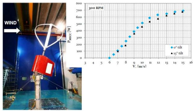
Figure 4.7.3 Left: DeepWind 1 kW rotor in high speed wind tunnel of Milan(I). Right: Power curves
