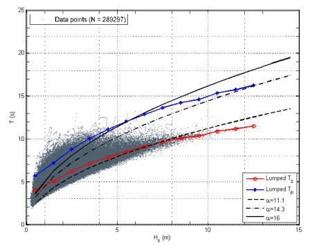
Figure 3.2.4 Hs - Tz scatter diagram of the mean wave periods and the lumped mean wave period and peak wave period. The black lines refer to equation (2.3,12) with different  $\alpha$ -values.
