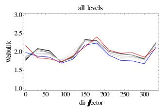
Figure 3.4.9. Similar to Figure .3.4.7, but for Weibull shape parameter k.
