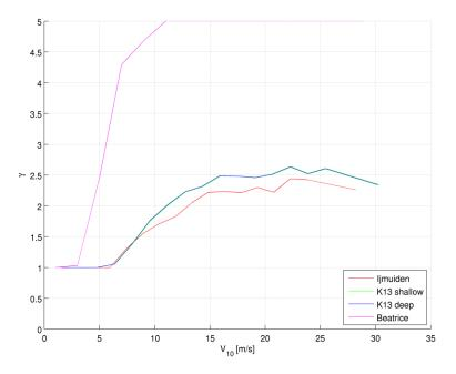
Figure 2.4.7 The peak factor  $\gamma$  versus the 10 meter wind speed for the 4 sites considered. The high values from Beatrice reflect the relatively low T<sub>p</sub> values for this site, see Figure 2.4.4.
