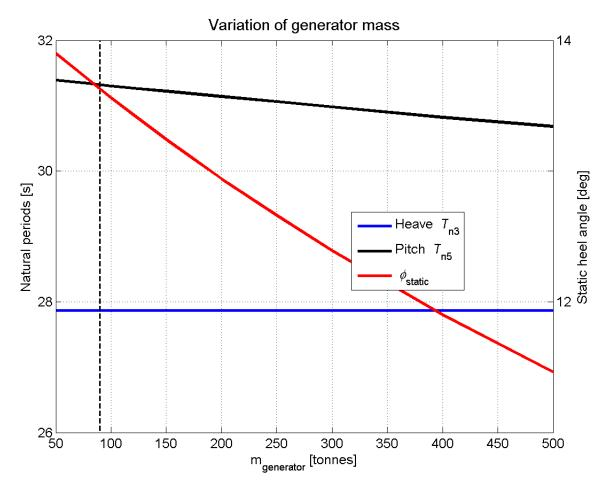
Figure 5.3.4 Effect of variation of generator mass on natural period and tilt angle
