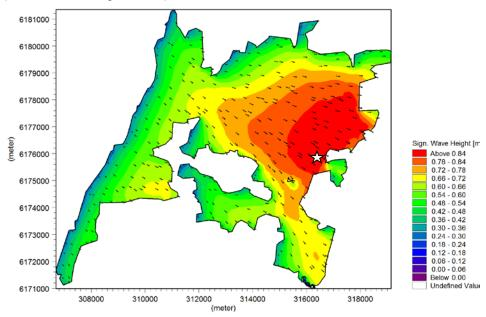
Figure 4.7.8 Wave height for wind speed of 20m/s from 300 deg N
