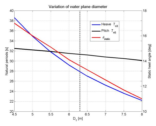
Figure 5.3.5 Effect of variation of diameter at SWL on natural period and tilt angle
