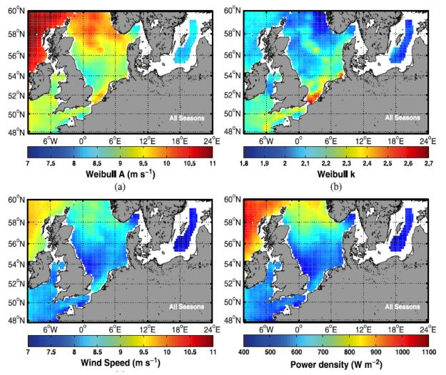
Figure 2.4.2 The 10 meter marine wind climate across the North Western European seas. The white areas correspond to lack of data, mainly due to precipitation. From [14].
