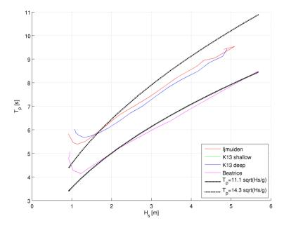
Figure 2.4.6  $T_p$  versus  $H_s$ , estimated from data at the four sites considered. For the UpWind sites (2), the data are tabulated in section 2.3. The Beatrice curve is from [10] and is on the lower bound, which may reflect the nearness of the coast at this site. The two analytical curves reflect bounds for  $T_p$  in (2.3.12).
