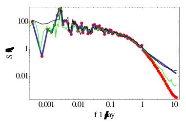
Figure 3.4.12. The power spectrum from WRF wind at 16.7 m (red), CFSR winds at 10 m (green) and a spectral model  $S(f)=a f^{5/3}$  for f>1 day<sup>-1</sup>(blue) and measurements from Utsira (black).
