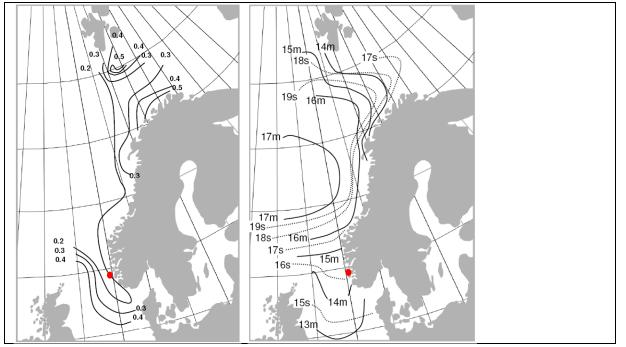
Figure 5.1.1 Maximum 100 year tidal surface current [m/s](left). Significant wave height Hs and related maximum peak period TP with annual probability of exceedance of  $10^{-2}$  for sea-states of 3 h duration. ISO-curves for wave heights are indicated with solid lines while wave period lines are dotted, maps from [[64.]].
