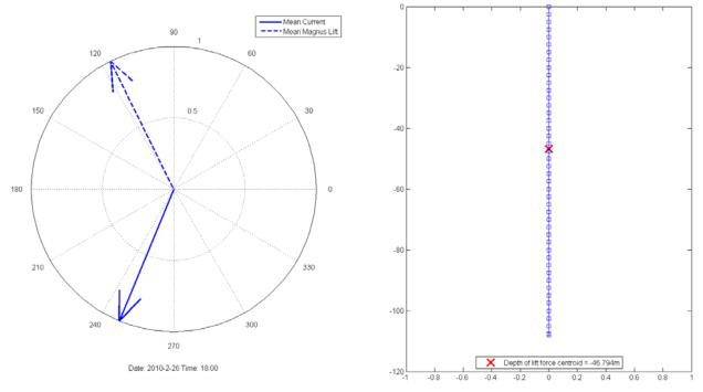
Figure 3.3.9 Normalised Mean Currents and Global Magnus Lift Force for 3 1-hour periods (3/3)
