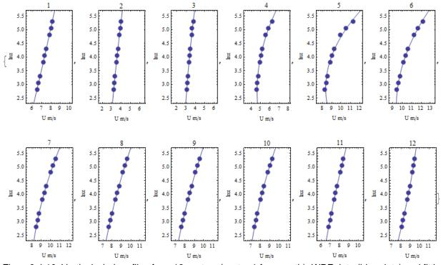
Figure 3.4.10. Vertical wind profiles from 12 sectors (sector 1 from north), WRF data (blue dots) and fitting (blue curves).
