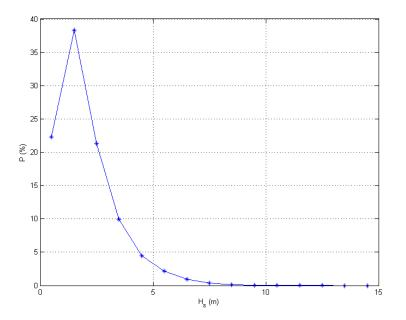
Figure 3.2.3 The probabilities of occurrence of the significant wave height.
