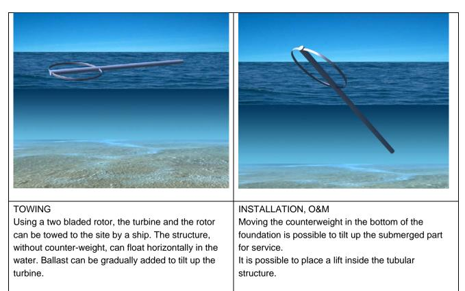
Figure 5.2.1 Artist view of concept under transport(left) and installation procedure(right)
