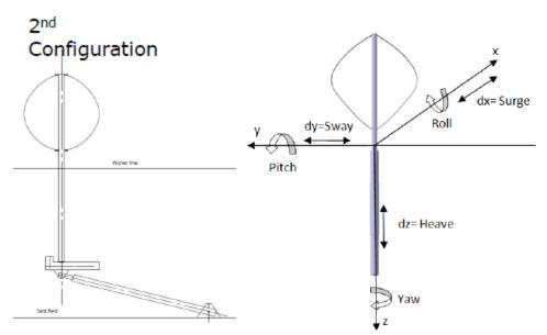
Figure 4.7.1 Left: Demonstrator heave, pitch, roll and yaw properties. Right: DOFs
