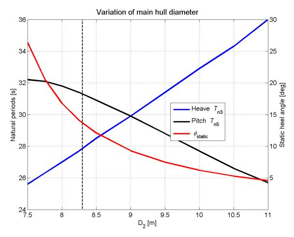
Figure 5.3.6 Effect of variation of main hull diameter on natural period and tilt angle
