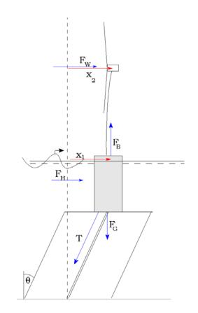
Figure 3.4.1. Model sketch for simple model of a TLP wind turbine.
