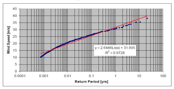
Figure 2.3.5. Extreme wind speed versus return period from UpWind IJmuiden data at hub-height. From [1].
