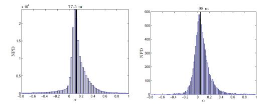
Figure 2.3.2. The shear power coefficient,  $\alpha$ , from two North Sea sites, Greater Gabbard and Beatrice. From [13].
