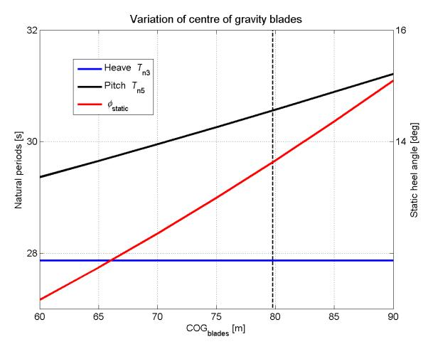
Figure 5.3.1 Effect of variation of COG of Blades on natural period and tilt angle
