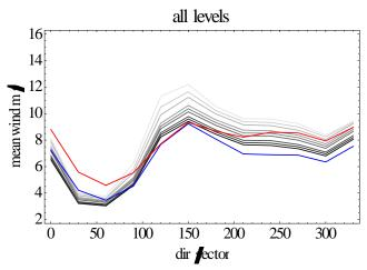
Figure 3.4.7. Mean wind speed in 12 sectors. Black-gray curves are WRF data from 16.7 m to 200.9 m. The blue curve is the CFSR data at 10 m. The red curve is the measurements from Utsira.
