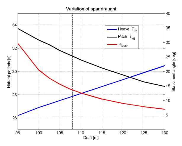
Figure 5.3.7 Effect of variation of floater draught on natural period and tilt angle
