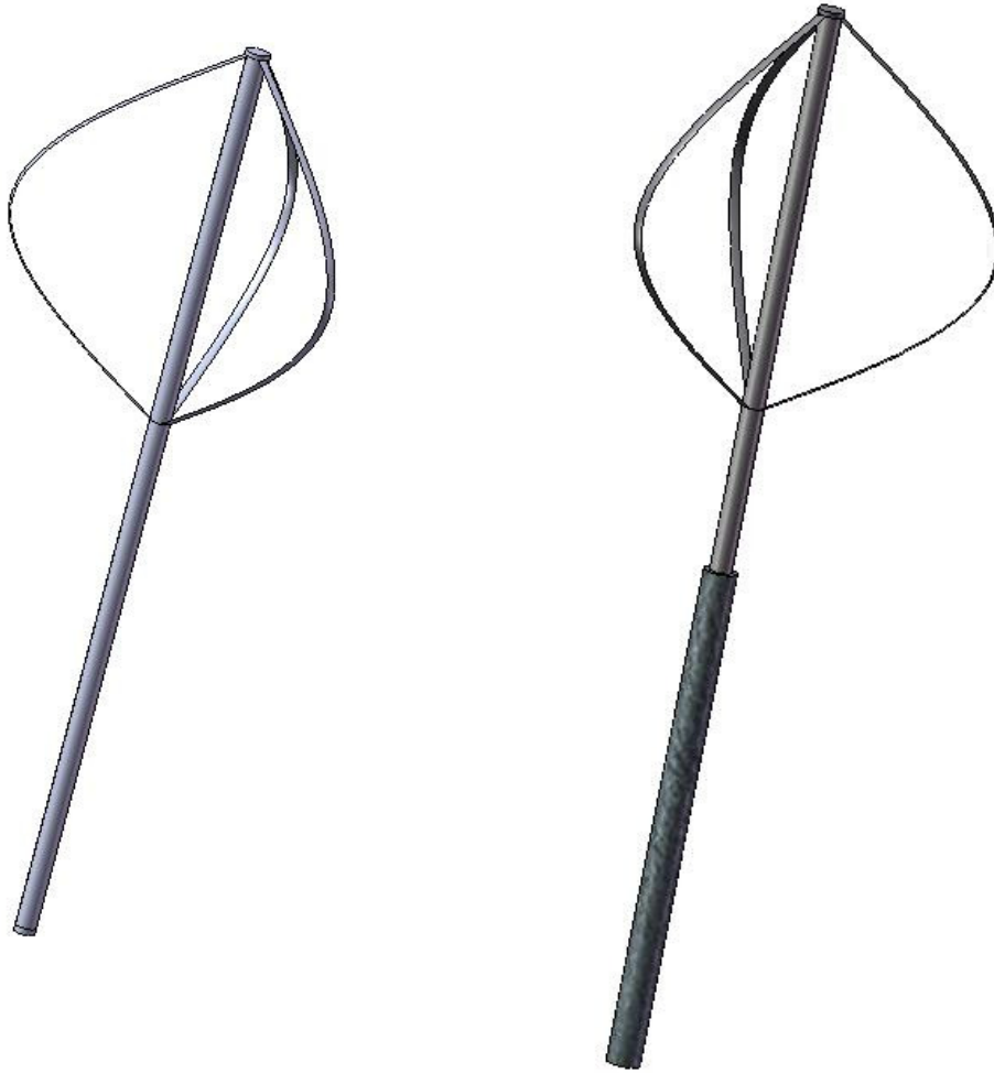
Figure 4.4.4 Drawing of the two main concepts: a. “all steel structure” b. steel structure with concrete foundation
