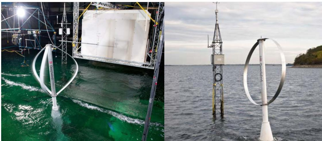
Figure 4.7.2 Left: Ocean lab testing of demonstrator at MARIN(NL). Right: Near to real tests in Roskilde fjord(DK)[78.]
