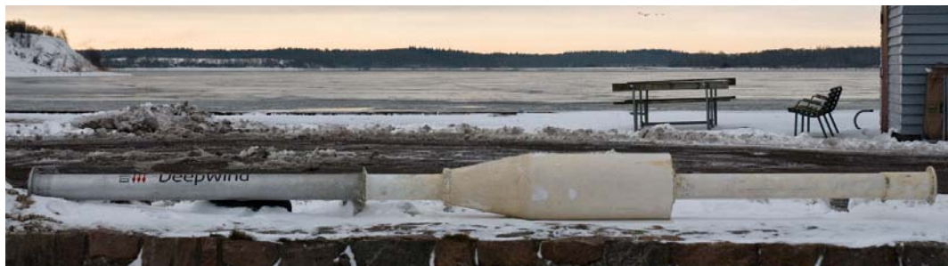
Figure 40 Rotor tube with buoyancy lying on the ground
