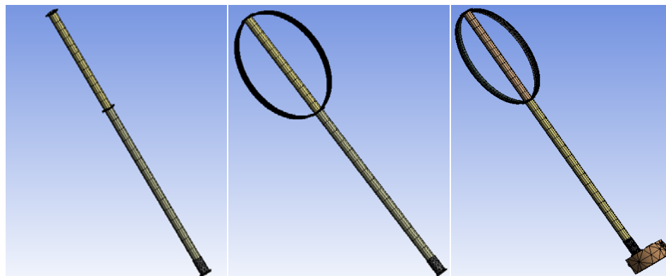
Figure 44 The three implemented FE models, tube alone, tube with two blades, tube with blades and generator box
