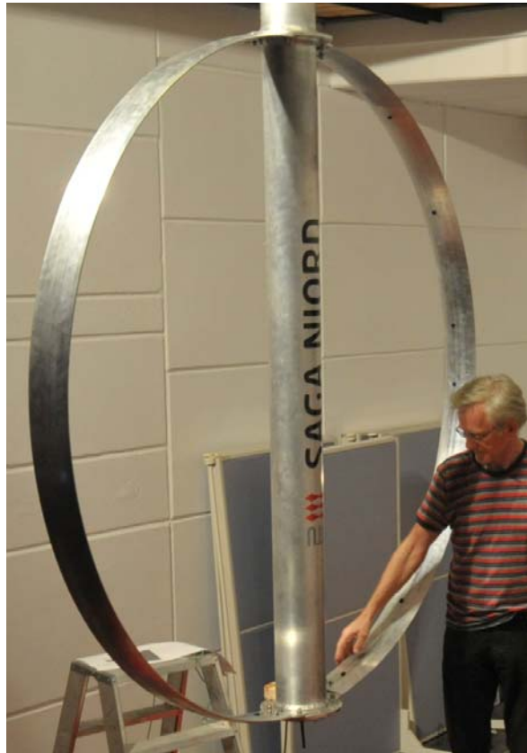
Figure 38 Windpower Tree blades mounted on the demonstrator rotor tube.
