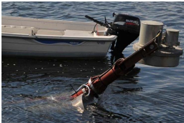
Figure 46: Rotatable support in gimbals joint of demonstrator generator on which the rotor is mounted on the right
