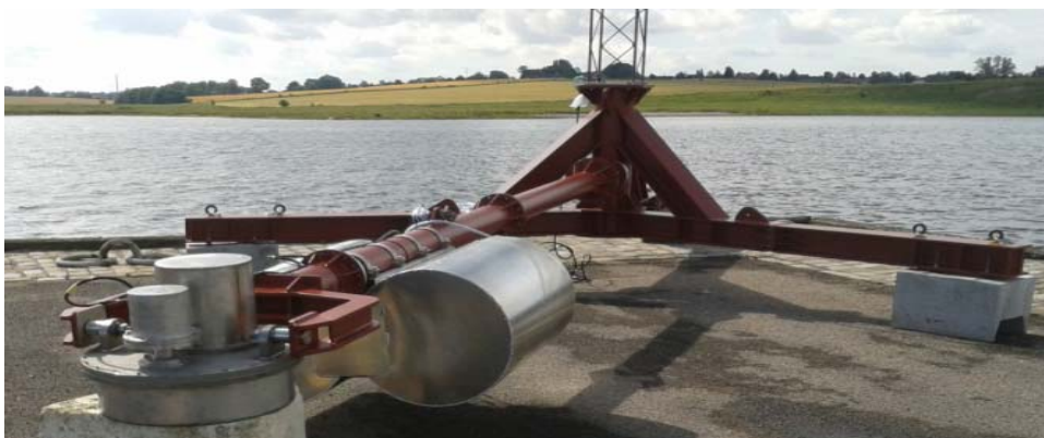
Figure 42 The foundation with concrete feet standing on the pier. On the torque arm the generator box and the air barrels are mounted.
