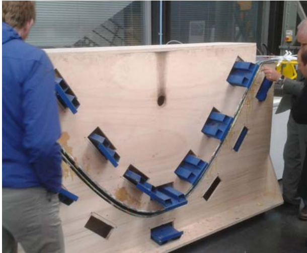
Fig. 35 Picture of mould for production of the GRP blades by Nanuphar
