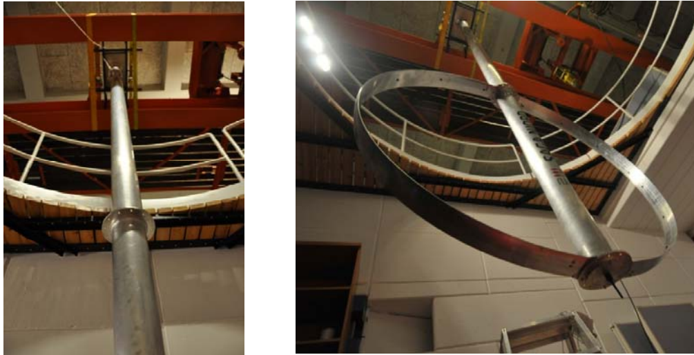
Figure 45: Setup of the experimental modal analysis of the tube alone (left) and the tube with blades (right).
