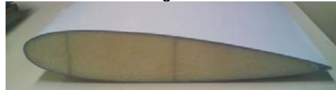
Fig 34 Profile structure of blades from Nanuphar (this profile is made for a larger blade)
