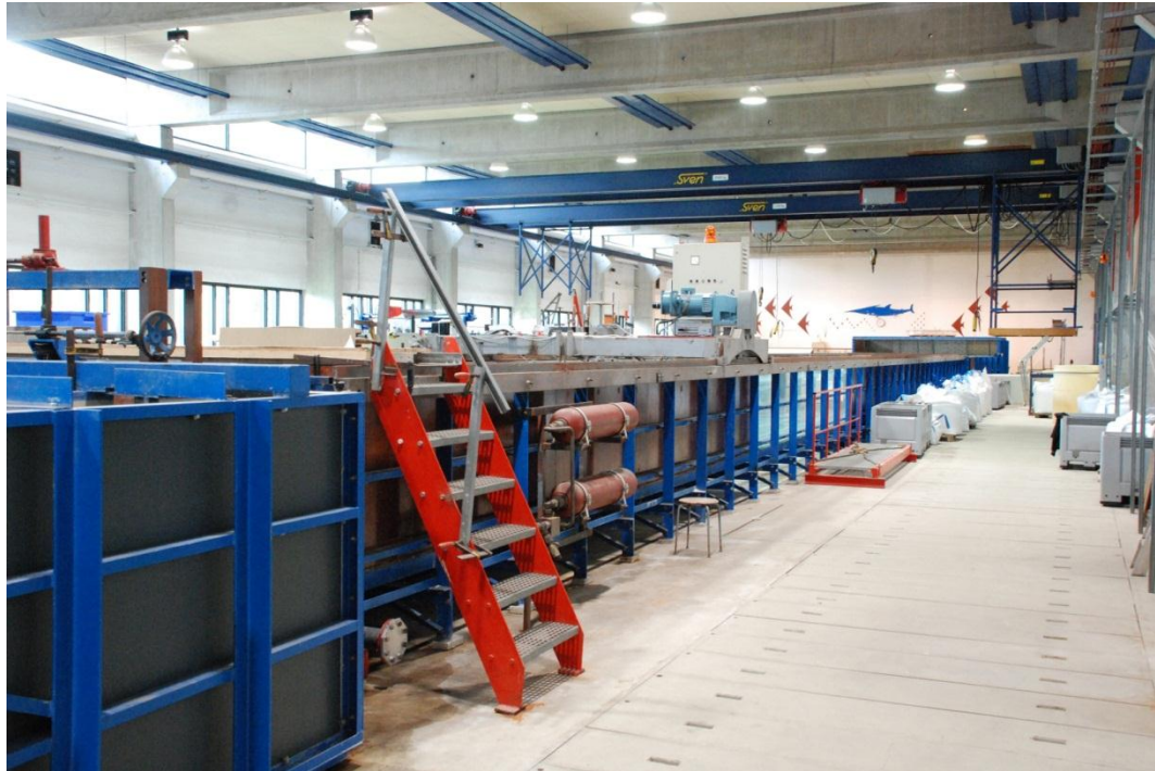
Figure 3.2 Current flume with carriage on top. The side walls are made of glass over a part of the measuring section allowing side view inspection.
