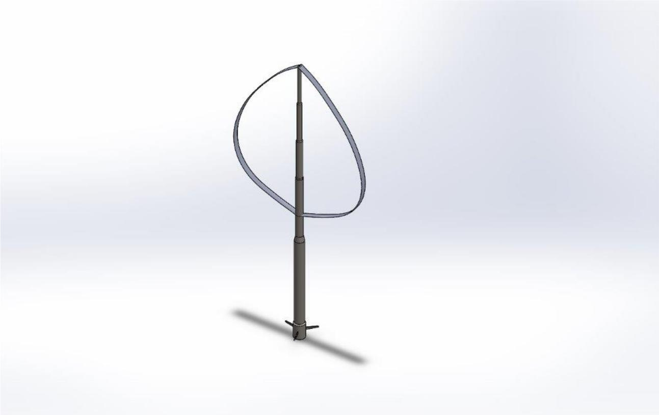
Figure 5.1.2 SolidWorks sketch of the 5 WM Baseline turbine©DTUWE
